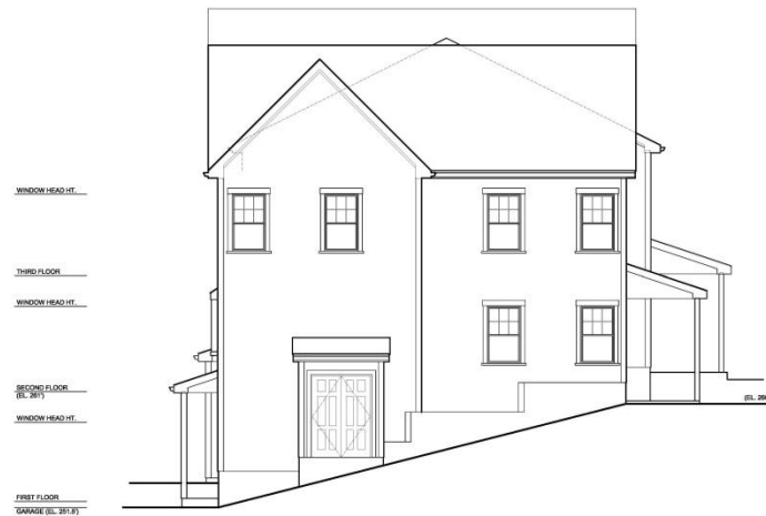
BUILDING TYPE TH4CDU - RIGHT ELEVATION 1 SCALE: 1/4"=1'-0"
