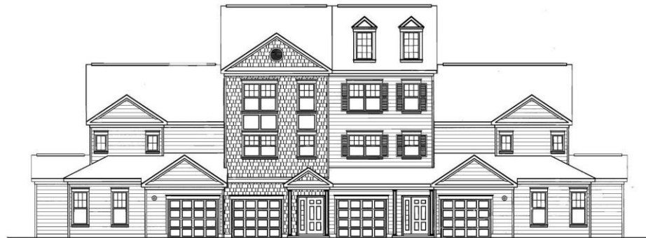
4 UNIT (A) - FRONT ELEVATION SCALE: 1/8" = 1'-0"
