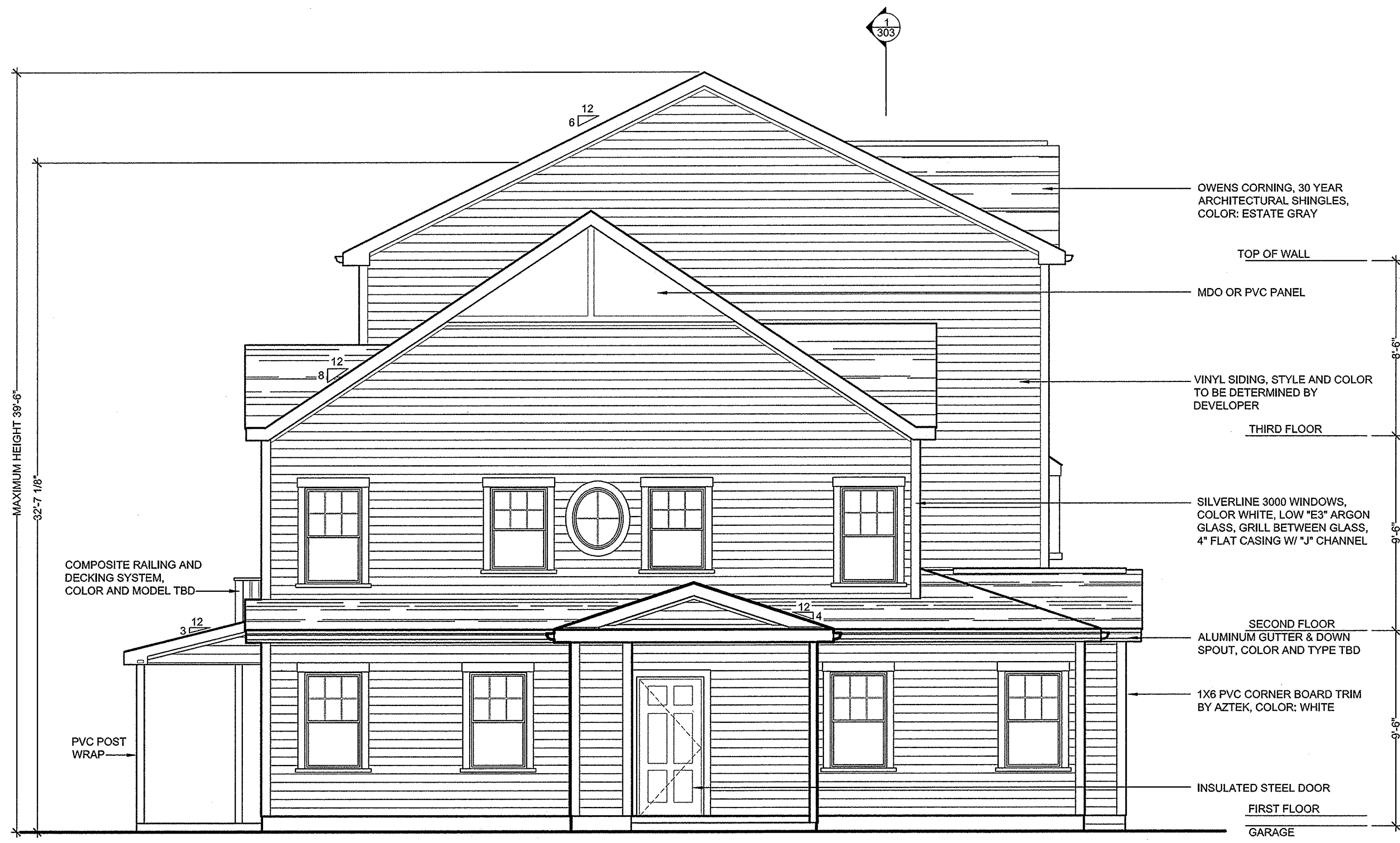
BUILDING TYPE TH4A3 - LEFT ELEVATION ① SCALE: 1/4"=1'-0"
