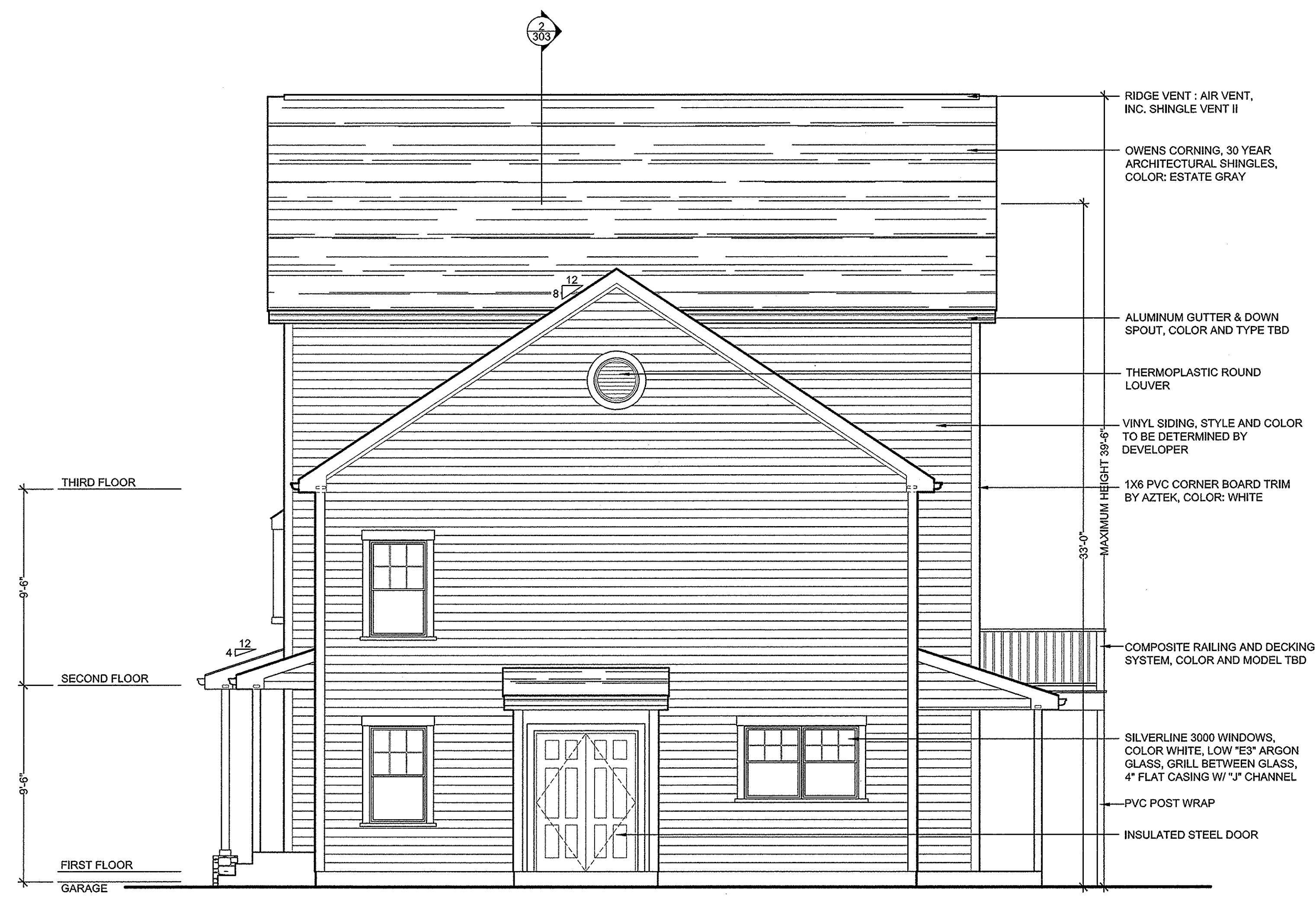
BUILDING TYPE TH3B3 - RIGHT ELEVATION ① SCALE: 1/4"=1'-0"
