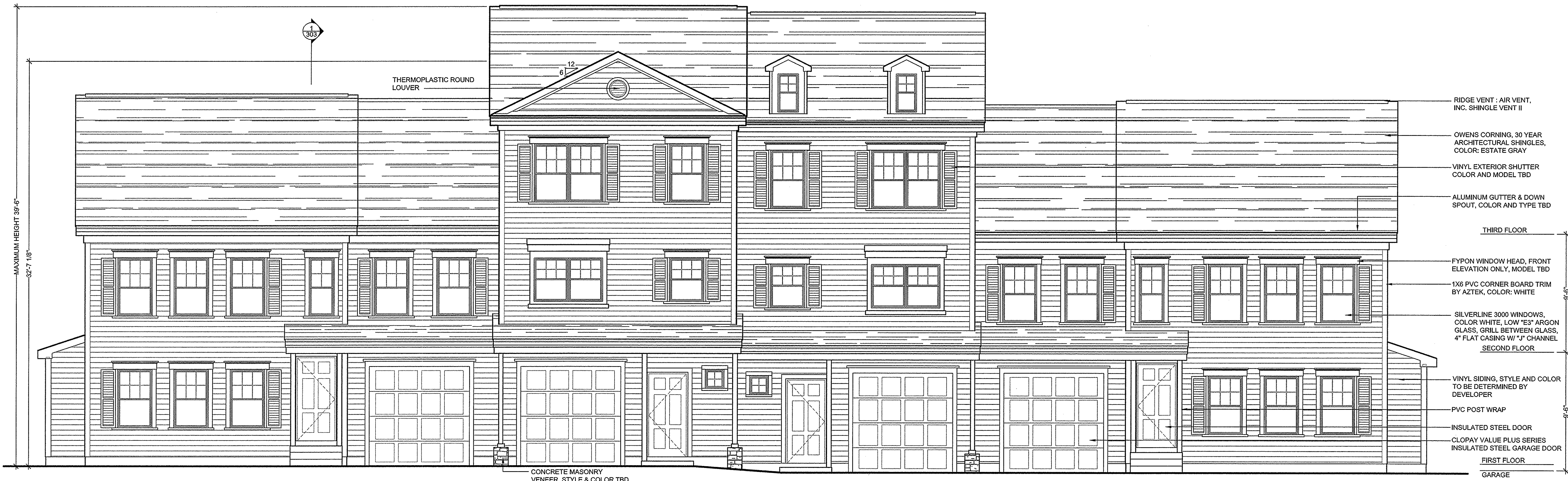
BUILDING TYPE TH4B3 - FRONT ELEVATION 2 SCALE: 1/4"=1'-0"
