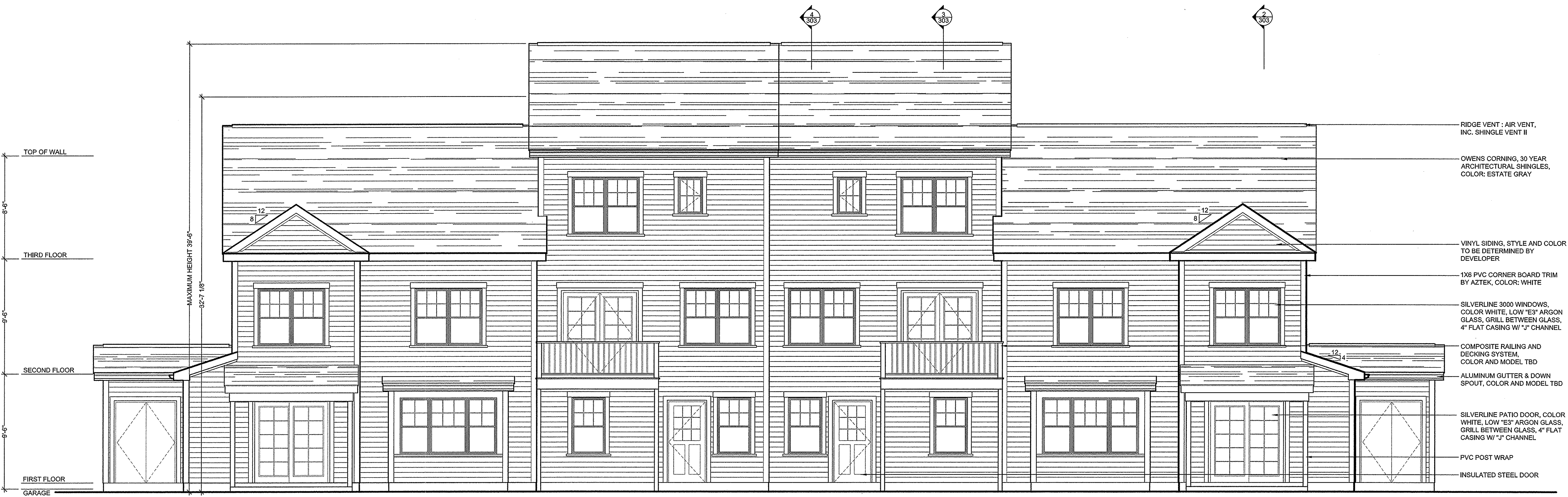
BUILDING TYPE TH4A3 - REAR ELEVATION ② SCALE: 1/4"=1'-0"
