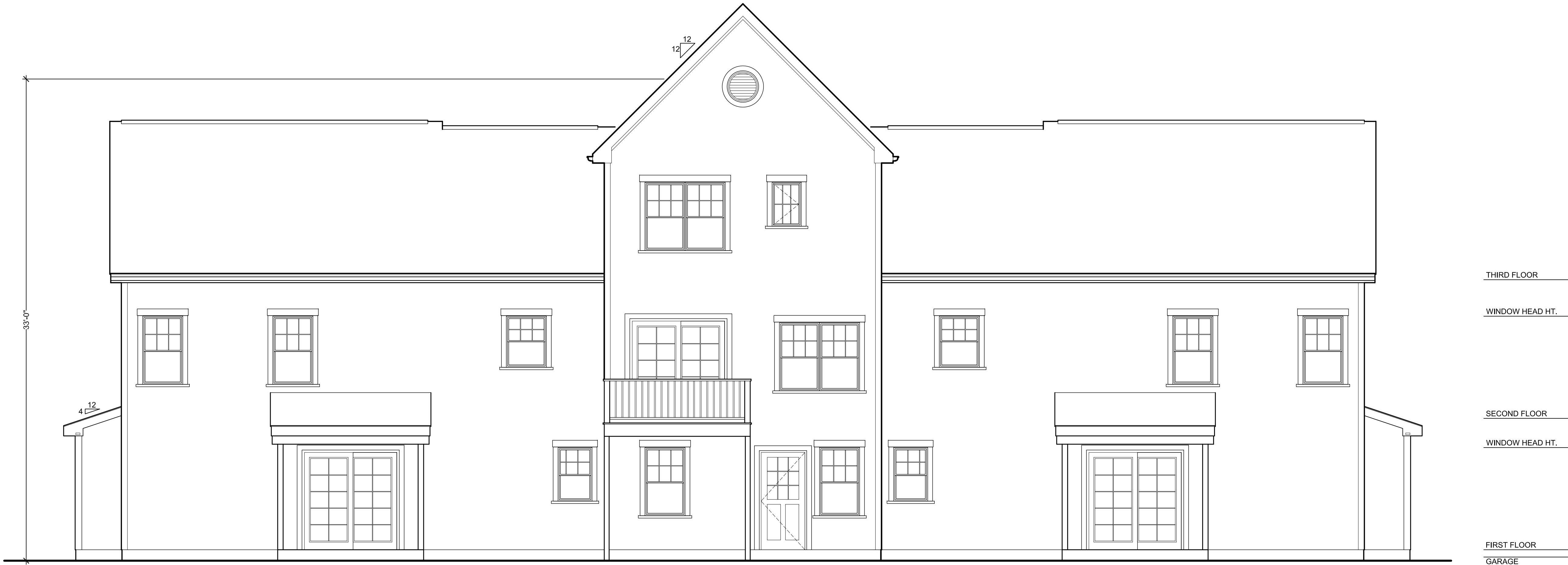
BUILDING TYPE TH3B3 - REAR ELEVATION 2 SCALE: 1/4"=1'-0"
