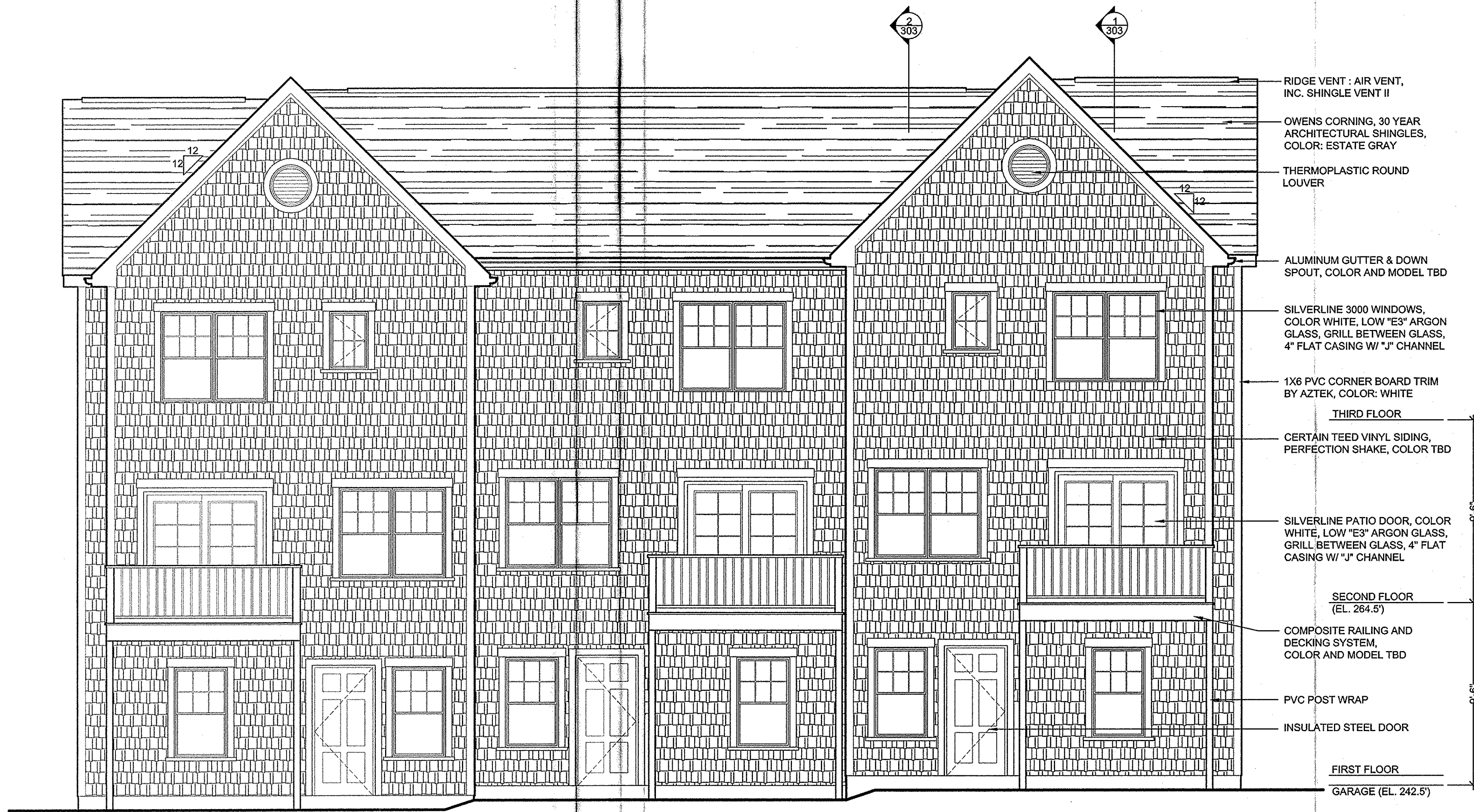
BUILDING TYPE TH3C - REAR ELEVATION
