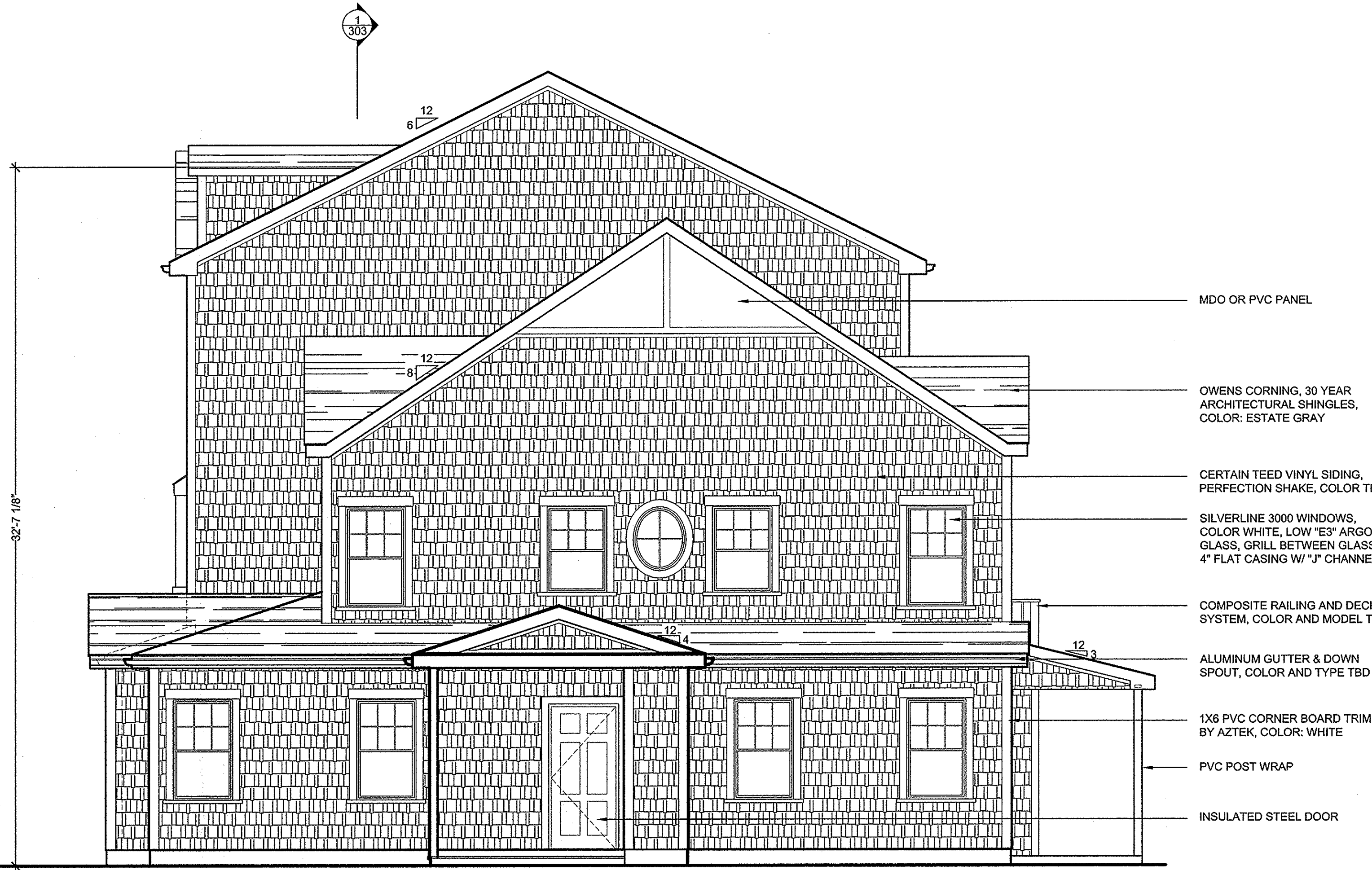
BUILDING TYPE TH4A3 - RIGHT ELEVATION
