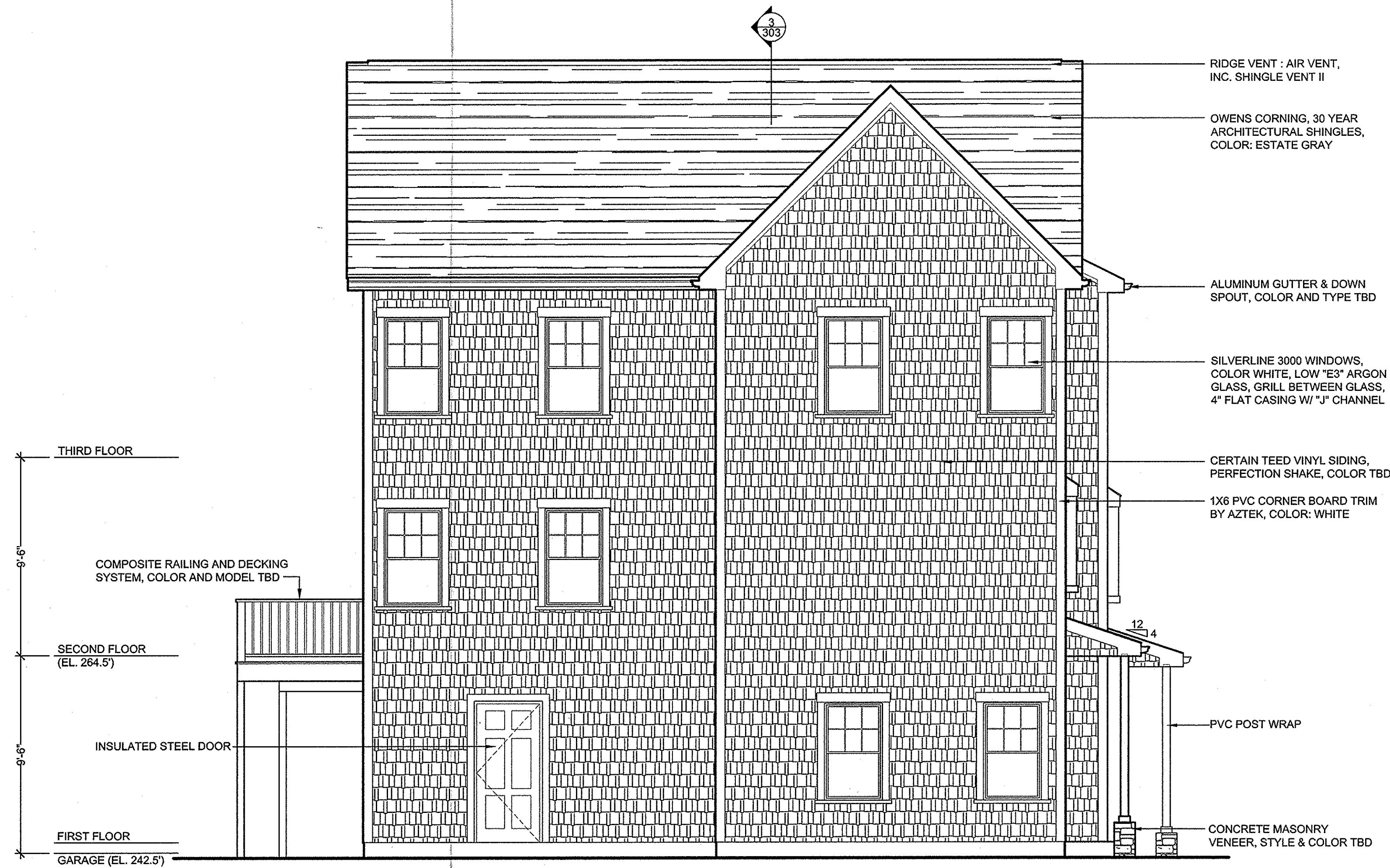
BUILDING TYPE TH3C - LEFT ELEVATION
