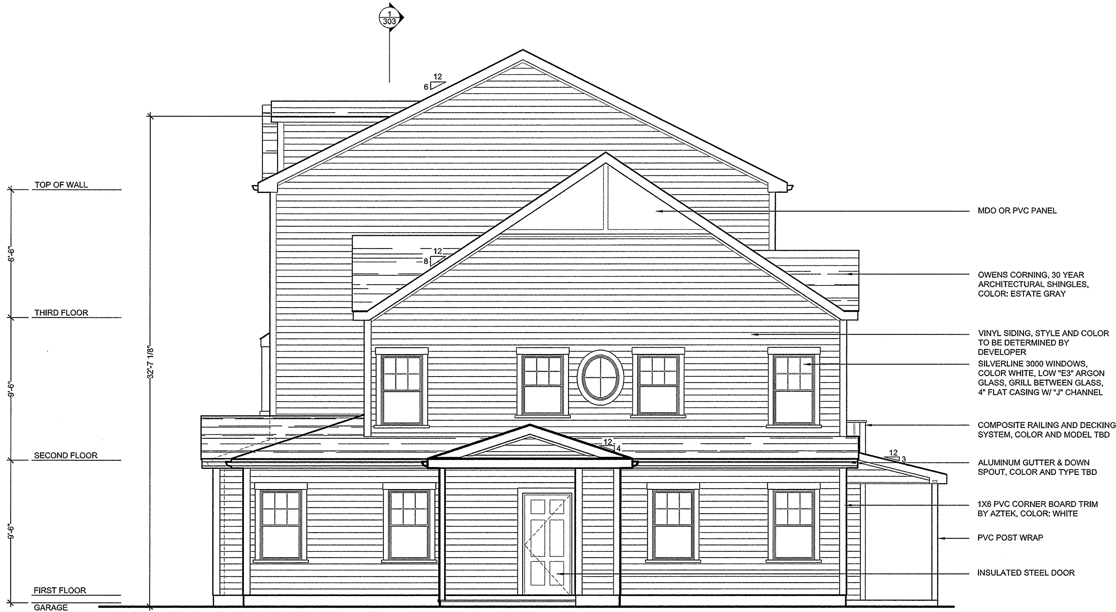
BUILDING TYPE TH4A3 - RIGHT ELEVATION
