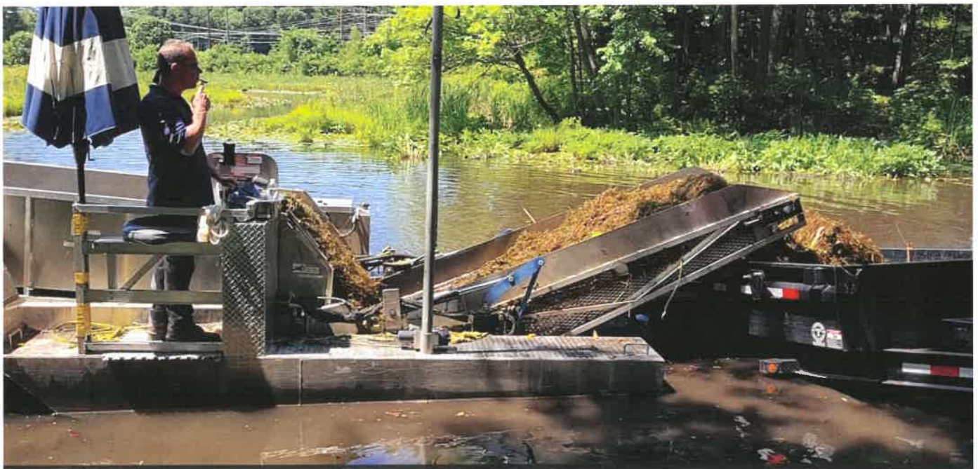
Figure 9 – Emptying the Eco-Harvester system using the conveyor belt to unload harvested plant material from the containment hopper into a trailer for removal.
