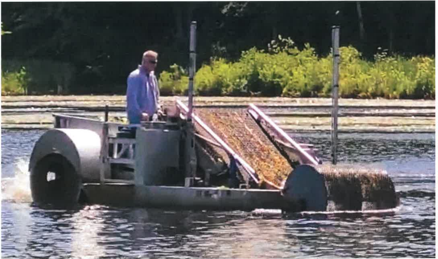
Figure 8 – Eco-Harvester system, showing overall vessel, rotating drum at the front, and conveyor belt carrying harvested plant material into the containment hopper.
