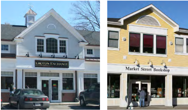
Wall signs should be scaled to fit the overall facade of the building. Most should be confined to a continuous horizontal sign band.
