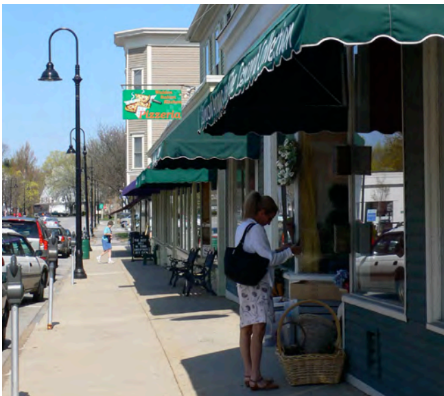
Adjustable awnings support sustainable building design by allowing users to adapt to changing weather and light conditions over the course of a day (or change of seasons) with minimal energy use.
