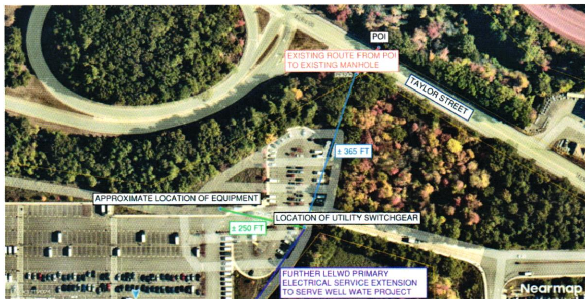
Figure E: Design Option #3 – Primary Service to feed EV Chargers from POI as part of Overall LELWD Primary Electrical Service Upgrade Project
