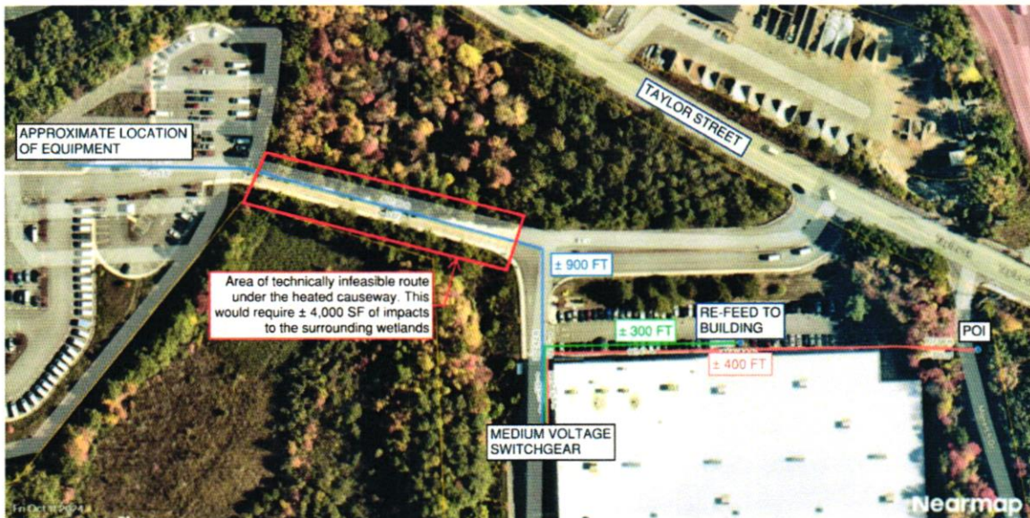
Figure A: Design Option #1 - Primary Service to feed EV Chargers and Building Loads
