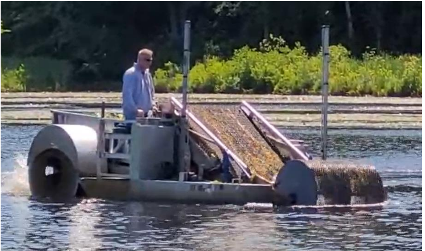
Figure 7. Eco-Harvester system, showing overall vessel, rotating drum at the front, and conveyor belt carrying harvested plant material into the containment hopper.
